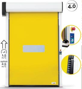
THE ZIP RAPID ROLL-UP DOOR is the most versatile of the Active range. The mantle provide with PVC zips, sliding on self-lubricating polyethylene guides and connect the sheet for the entire height of the door ensuring water tightness and wind resistance (class 3). The ZIP doors are self-repairing up to a width of 4000 mm.
